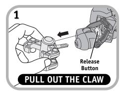
Press the release button on URV's arm.
