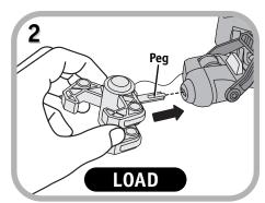
• Insert the peg on the claw into the hole in the arm. Press the claw until it locks in place.
