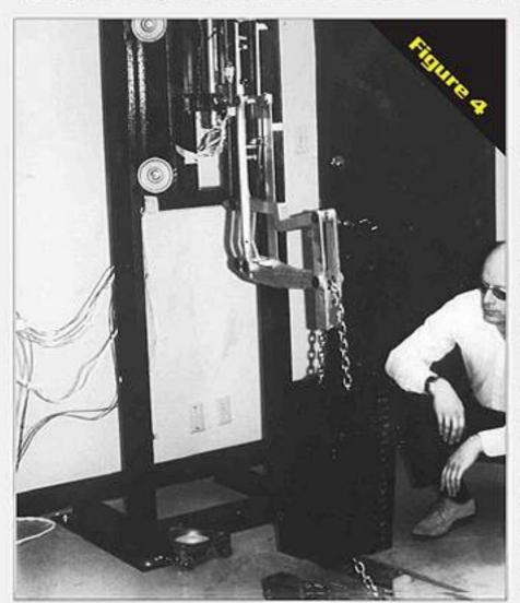
it is amazing that the robot only required 450 watts in active mode and 2 watts in the stand-by mode. For the initial concept demonstrator, the aircraft battery supplied all the power Steve required. Even so, the battery had to be recharged after an hour's use. Later versions used different batteries and these different chemistries brought greater capacities.
