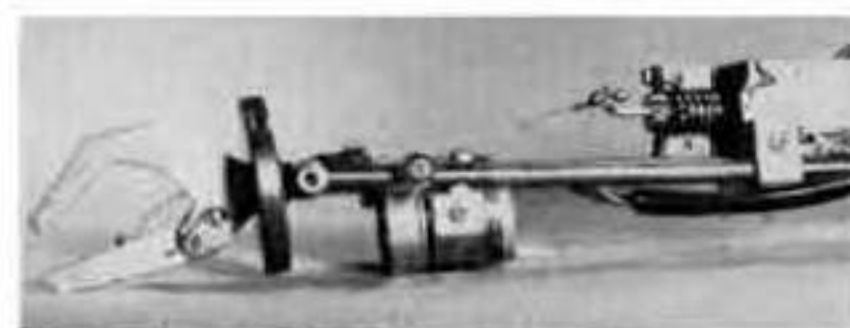
FIG. 56—COMPLETED rotatable end-effector mounted on forearm shows modified connection to solenoid using solid steel wire.
