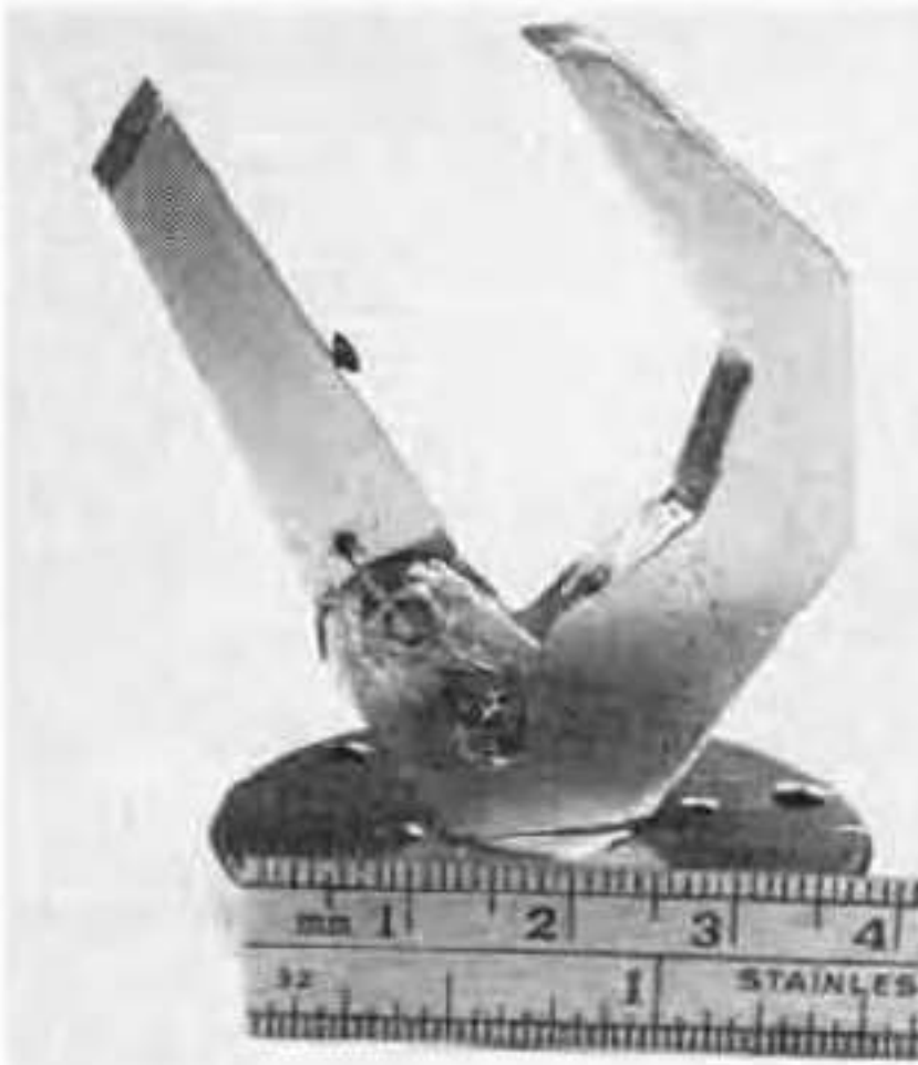
FIG. 16—CLAW-TYPE end-effector showing homemade torsion spring. Text gives details.
