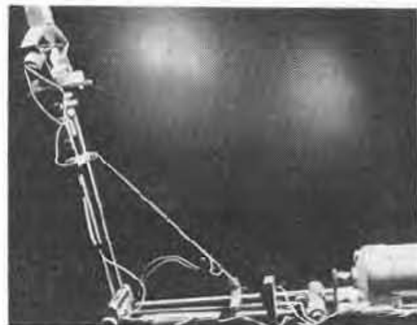
FIG. 9—MANIPULATOR, showing contractor-bar and its attachment to the two pivot-pieces.
