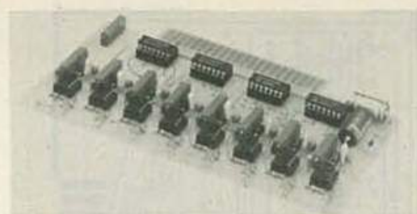
FIG. 79—WHEN MOUNTING POTENTIOMETERS make certain to allow clearance between them and IC sockets for screwdriver adjustment.
