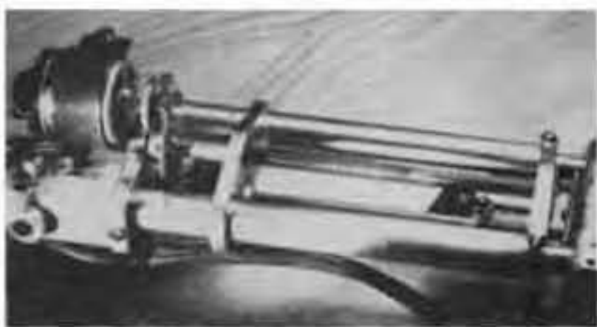
FIG. 63—COMPLETED EXTENDER ARM shows how new motor is attached and how it is connected to drive threaded rod.
