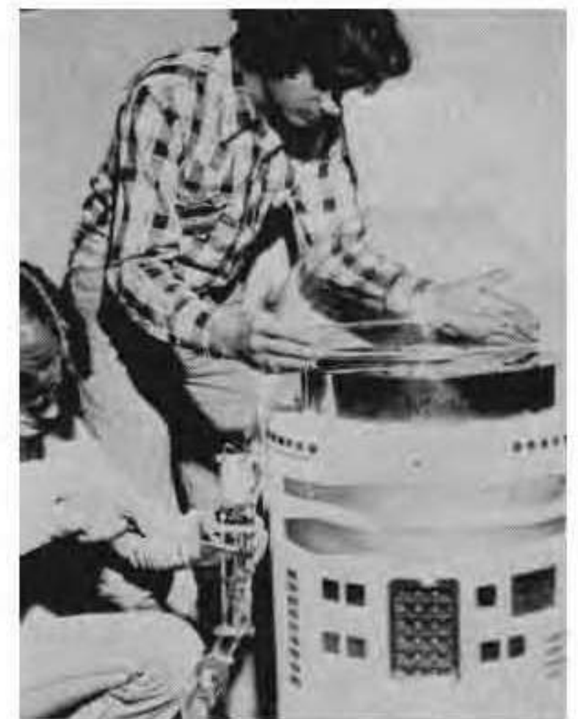
FIG. 41—ROBOT'S DOME can be made from salad-spinner or from terrarium cover.
